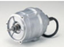
**High-Performance Motor:** Dry type, squirrel-cage, induction motor, housed in a watertight casing, conforms to either insulation class B or E, or F. In both of these classes, all standard pumps can be used in ambient temperature up to 104°F (40°C).
