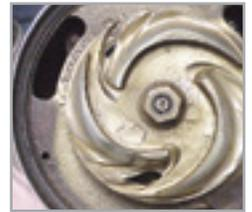
Competitor Impeller is effectively worn out.
