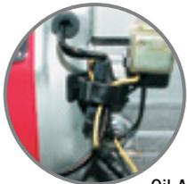
Oil Alert System **automatically shuts the engine down** if the oil level falls below the safe operating level.
