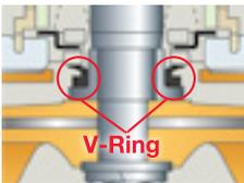
**V-Ring:** V-Ring is mounted at the top of the impeller and is brought in close contact to the bottom of the mechanical seal by the internal pressure of the pump casing. This V-Ring acts as a dust seal to prevent fine abrasive particles in the pumping fluid from reaching the mechanical seal.
