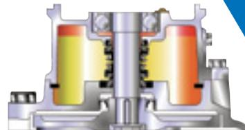
**Oil Lifter:** Tsurumi's Oil Lifter encloses the mechanical seal and uses the centrifugal force generated by the rotating shaft and seal to pump oil to the upper seal faces. Upper and lower seal faces are positively lubricated even when extremely low oil levels exist, as experienced after long periods of extended operation.
